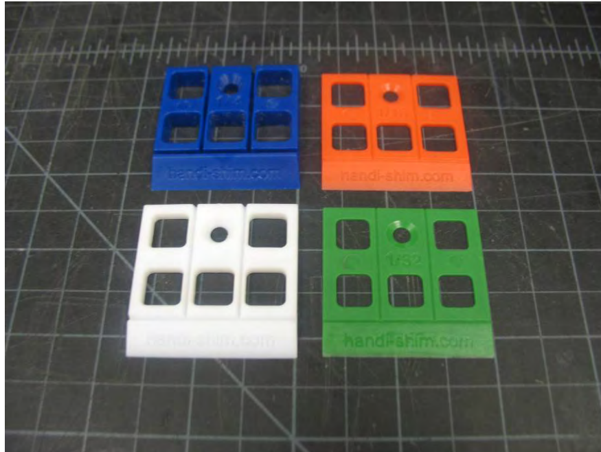
Photo No. 1 Complete Handi-Shim Sample Series - Pre-Test Condition (Top to Bottom, Left to Right: 1/4 in, 1/8 in, 1/16 in, and 1/32 in)
